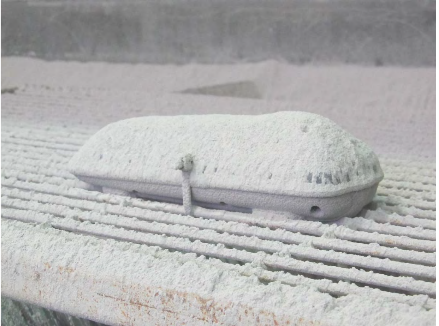
SPECIMEN TRAC STORES NUMBER TRA-0106769-S1 IN DUST CHAMBER AFTER TESTING
