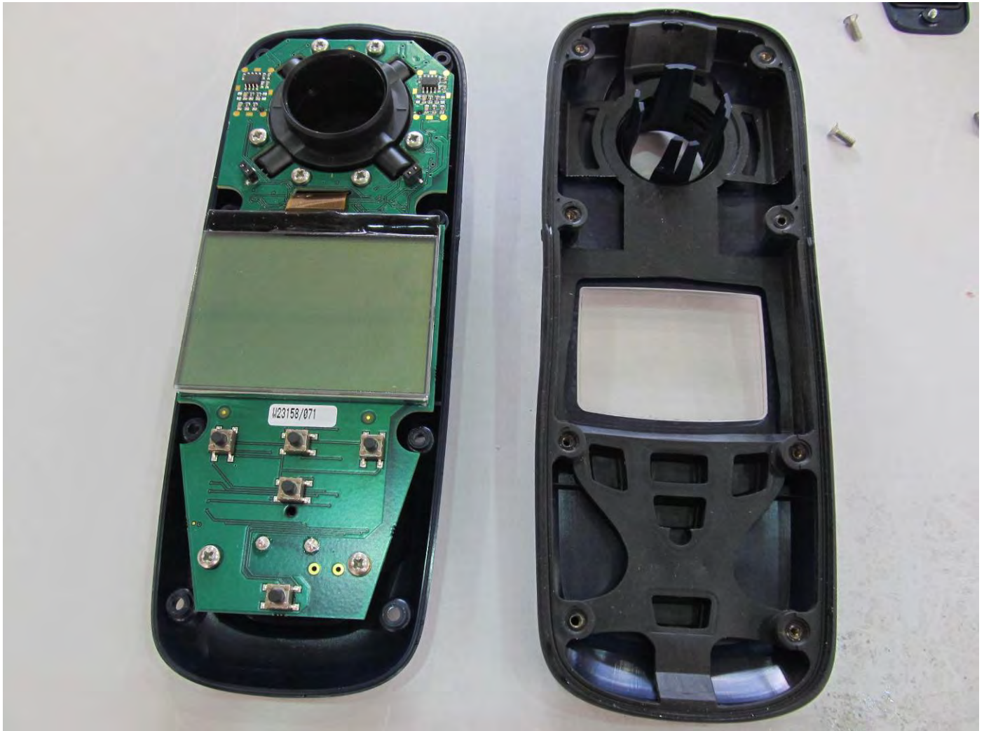
INTERNAL INSPECTION AFTER IMMERSION TEST
