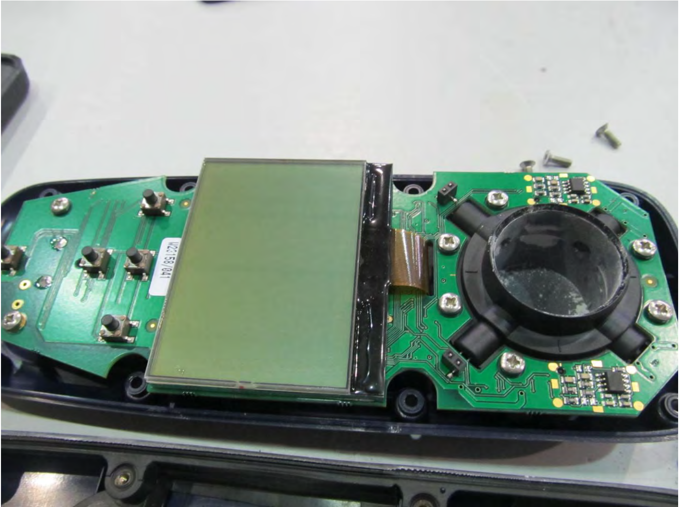
INTERNAL INSPECTION AFTER DUST TEST
